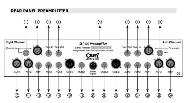
**Special Note:** The balanced input and output XLR connectors follow the ITT Cannon pin out configuration. This pin-out calls for the shield to be wired to pin #1. The normal- phase (hot) is wired to pin #2. Pin #3 is the inverted phase.
